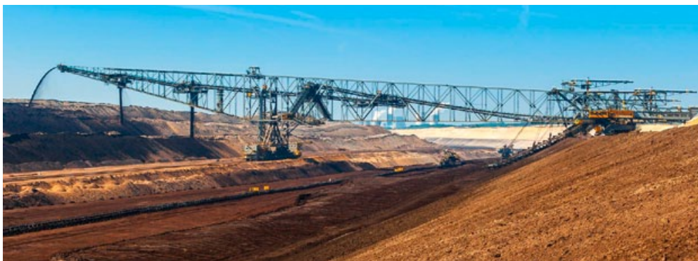
Illustration 2: Jänschwalde/ Cottbus North spoil conveyor bridge in the opencast brown coal mining
